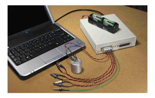
The red / green twisted pairs are differential inputs for each of the four analog channels. The black wire is AGND, which is not required for a floating sensor. Digital IO and GPS connections are available on the right front panel DB25. The USB8CH can be powered from eight AA rechargeable batteries for over 20 hours. A wide variety of other DC power supplies are also acceptable. Below is a screen shot of the Scope Windows application.
