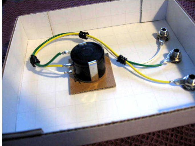
Figure 10.9: 10 turn potentiometer, reverse side connections
