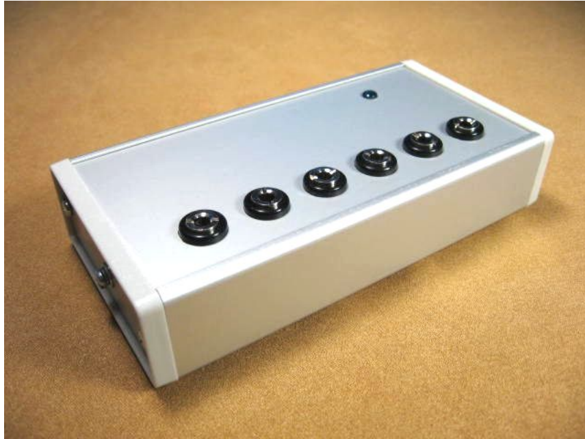
Figure 2.1: VREF-399 banana jacks with low voltage on the left / high on right
