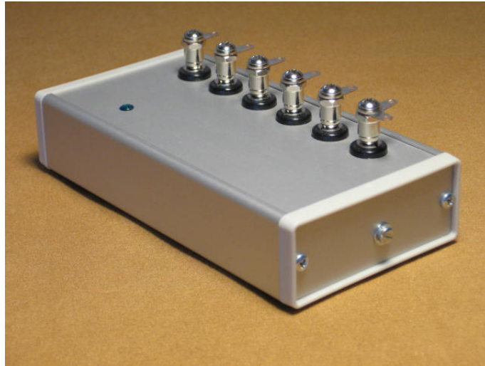
Figure 7.1: VREF-399 with banana plugs installed
