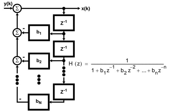
FIGURE 14B. IIR FILTER BLOCK DIAGRAM
