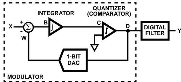
FIGURE 1. FIRST ORDER SIGMA DELTA ADC BLOCK DIAGRAM
