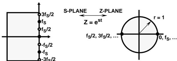
FIGURE 12. S PLANE AND Z PLANE MAPPING
