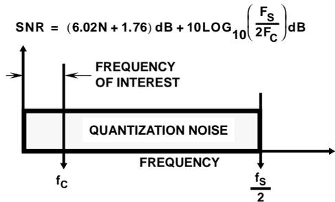
FIGURE 7B. OVERSAMPLED CONVERTER QUANTIZATION NOISE SPECTRUM
