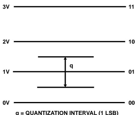
FIGURE 3. CODE EXAMPLE OF A 2-BIT A/D CONVERTER
