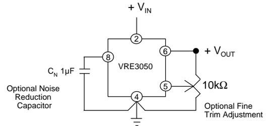
Figure 3 External Connections
